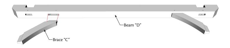
**Step 2:** Slide Post "B-1" & "B-2" into Beam "D" and simultaneously slide Brace "C" into Post "B".
