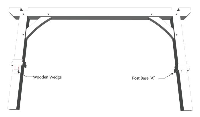
**Step 5:** Lift eave side of pavillion either manually or with a lift after steps 1-4 are completed and set on prepared concrete pad or wooden floor. Put temporary bracing in place to keep side from falling over until Step 6 is complete.
