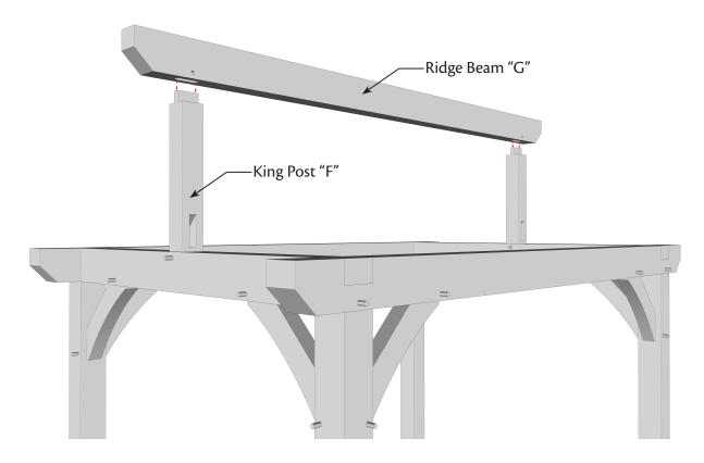
**Step 10:** Slide Gable Brace "H" into King Post "F" and simultaneously lower Gable Rafter "I" on top of Gable Brace "H". Make sure Gable Rafter "I" is securely down on top of beam. Follow Steps 10-A & 10-B after installing each gable rafter.
