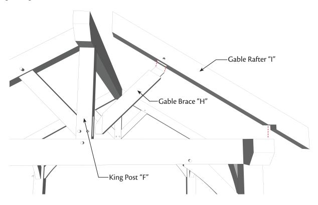
**Step 10–A:** Fasten the bottom of each Gable Rafter "I" with two 6" GRK screws and fasten the bottom of each Rafter "J" with one 6" GRK screw.
