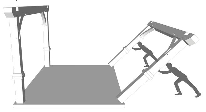
**Step 6:** Lower Beam "E" down into the notch in Beam "D" and simultaneously slide Brace "C" into Post B-1 & B-2 and also Beam "E" at the same time. After beams and braces are installed, repeat step 3 with all the required pegs.
