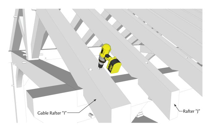
**Step 10–B:** Fasten the top of each Gable Rafter "I" with two 6" GRK screws and fasten the top of each Rafter "J" with one 6" GRK screw.
