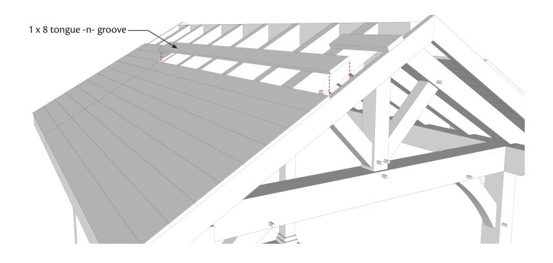
**Step 15:** After all decking is installed, add 1 x 3 roof purlins for metal roofing. Purlins will be 24" o.c. for ag Metal and 16"o.c. for standing seam metal. Fasten with two nails into each rafter.
