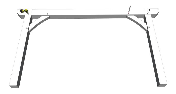
**Step 4:** Slide Post Base "A" approximately 30 inches up over the post, and put in a wooden wedge to keep post base from sliding down.
