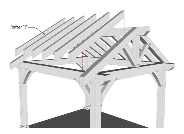
**Step 12:** Fasten 2 x 6 guttter board to each rafter with two nails.
