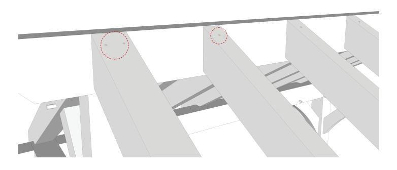
**Step 11:** Install Rafter "J" according to blueprint rafter spacing and make sure rafters are securely down on top of beam. Follow Steps 10-A & 10-B after installing each rafter.
