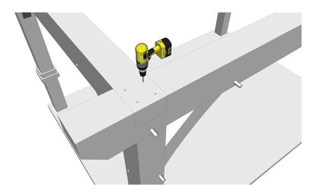
**Step 7:** Before proceeding, make sure the building is completely square. Then fasten the post to the floor with the included Simpson angle brackets and screws (a tapcon will be needed). There will be two brackets per post, and brackets should always be on the insides of posts. After brackets are installed, remove wedge and let post base slide to bottom of post.
