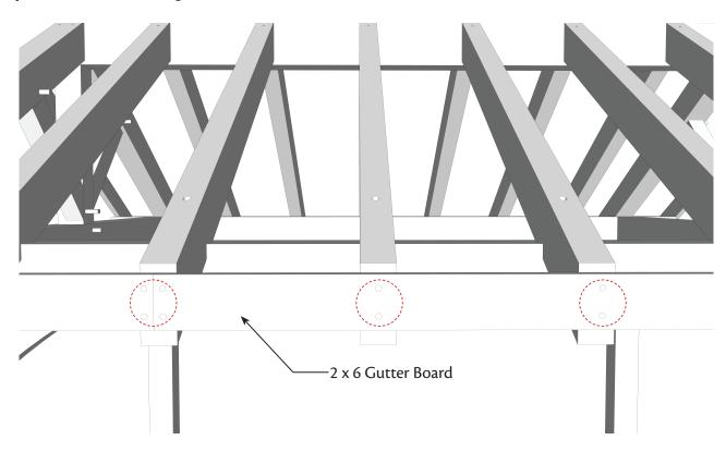
**Step 13:** Add 2 x 6 gable faceboard and fasten bottom to gutter board with two nails. Add a temporary 2x blocking from top of gable rafter to top of gable faceboard. Blocking supports gable faceboard until 1 x 8 tongue-and-groove is installed. See Step 14 to see when blocking is removed.
