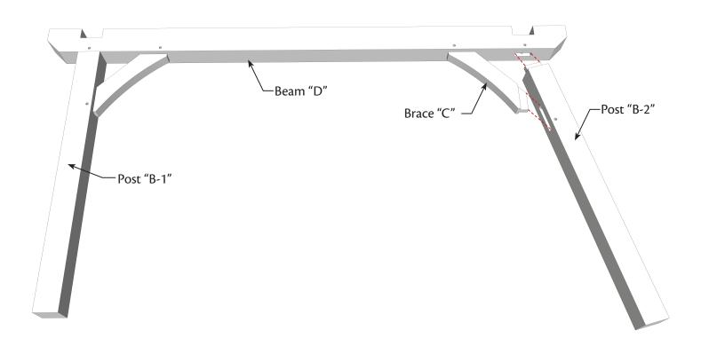
**Step 3:** Make sure posts and braces fit securely in beam. Drill a hole through post and brace, then hammer the pegs into the holes using a rubber mallet.
