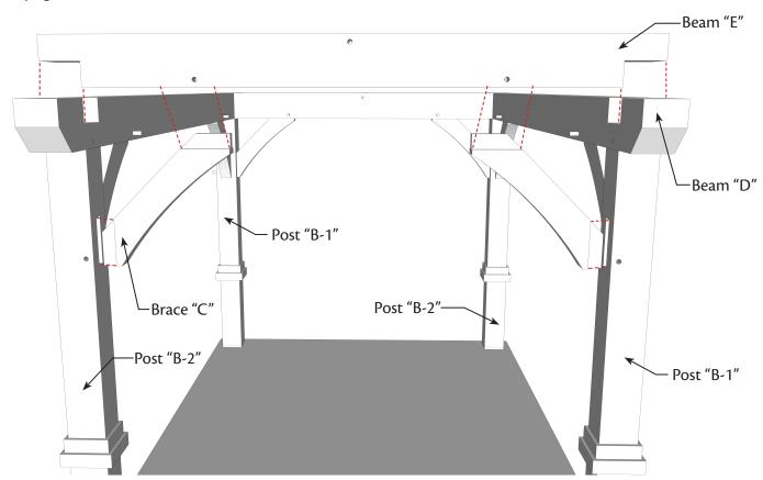
**Step 6-A:** Attach Beam "E" to Beam "D" with the included 8" GRK screws using four per side.
