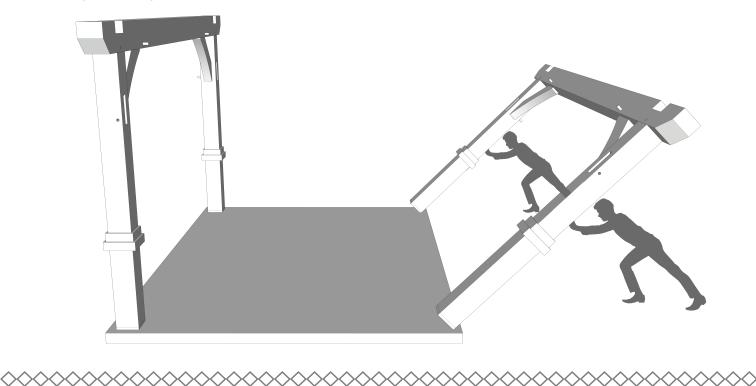
**Step 6:** Lower Beam "E" down into the notch in Beam "D" and simultaneously slide Brace "C-2" into Post B-1 & B-2 and also Beam "E" at the same time. After beams and braces are installed, repeat step 3 with all the required pegs.
