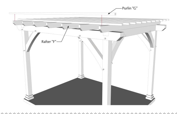
**Step 11:** Fasten each Purlin "G" to each rafter below with one 3 1/2" screw per rafter.
