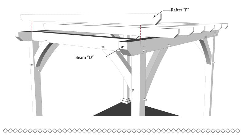
**Step 9:** Fasten each Rafter "F" to beam below with one 6" GRK screw on each side.
