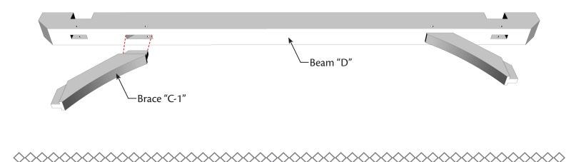
**Step 2:** Slide Post "B-1" & "B-2" into Beam "D" and simultaneously slide Brace "C-1" into Post "B".
