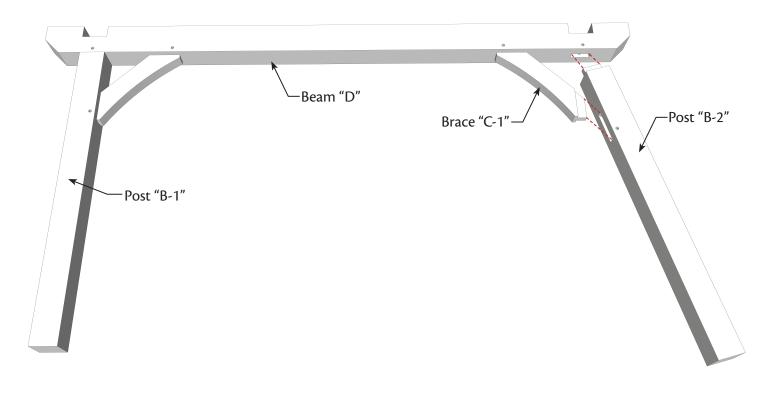
**Step 3:** Make sure posts and braces are securely in beam. Drill a hole through post and brace, then hammer the pegs into the holes using a rubber mallet.
