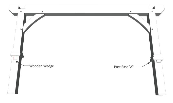
**Step 5:** Lift eave side of pergola either manually or with a lift after steps 1-4 are completed and set on prepared concrete pad or wooden floor. Put temporary bracing in place to keep the side from falling over until Step 6 is complete.
