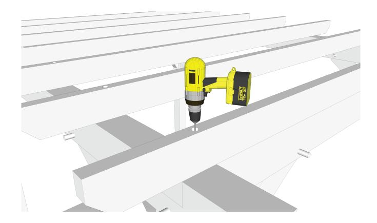
**Step 10:** Lower Purlin "G" down on top of Rafter "F" according to blueprint purlin spacing.
