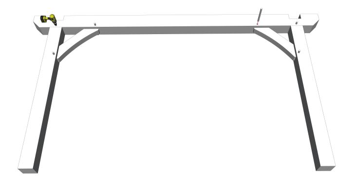
**Step 4:** Slide Post Base "A" approximately 30 inches up over the post, and put in a wooden wedge to keep post base from sliding down.
